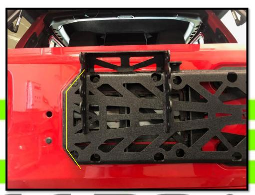
10. Remove the factory third brake light from original tire carrier by removing the (4) screws.
