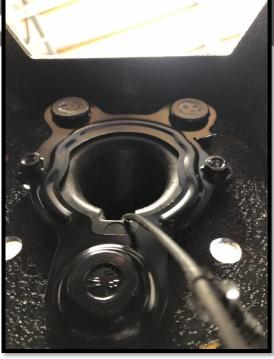
15. Using the provided camera enclosure, cover the camera and bolt using supplied flush mount allen head bolts.
