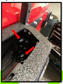
18. Tighten down (4) four tire mount bolts. Ensure all hardware is secure. Install plastic bumps on side of carrier.
