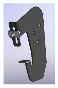
Place the rocker panel bracket assembly up to the plug hole locations in the rocker panel. Slide the threaded plate into plug holes. Center the threaded plate in the hole and then tighten the bolt using a 9/16" wrench / or socket. (Front and Middle Locations Only)
