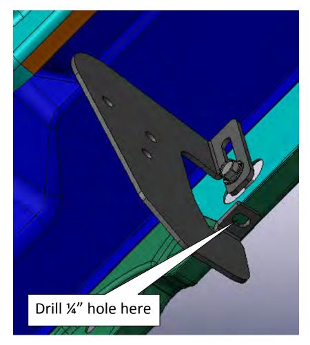
Secure the bottom of the rocker panel bracket to the rocker panel lip using a  $\frac{1}{4}$ " x 1" ribneck carriage head bolt (J),  $\frac{1}{4}$ " flat washer (K), and  $\frac{1}{4}$ " hex nut (L). Tighten into place using a  $\frac{7}{16}$ " wrench / or socket.
