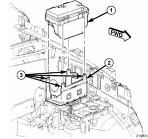
8. Disconnect each of the seven TIPM wire harness connectors from the TIPM housing. NOTE: Take care when removing the connectors.
