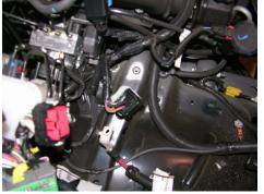
12. Remove the axle vent tube and ground wire from the 2 strut studs.
