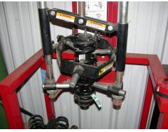
26. Remove the dust cover and washer from strut shaft.
