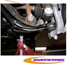
19. Remove the lower bolt at the lower control arm securing the clevis bracket with a 24mm socket.
