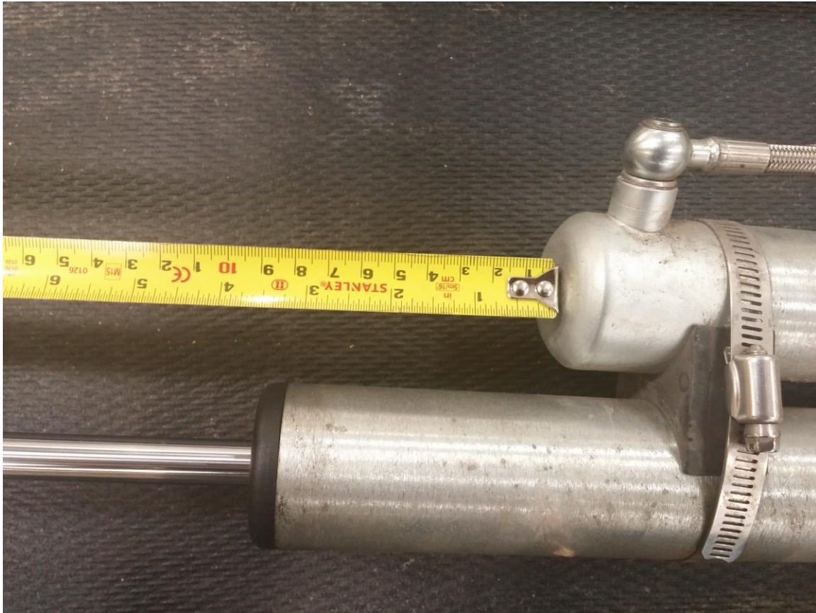
Figure 2. Reservoir placement in relation to end of main tube. Reservoir end should be about 3.5"-4" from end of main tube.
