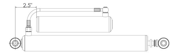
Figure 2. Reservoir placement in relation to Eye Ring. Reservoir end should be about 2.5" from Eye Ring.
