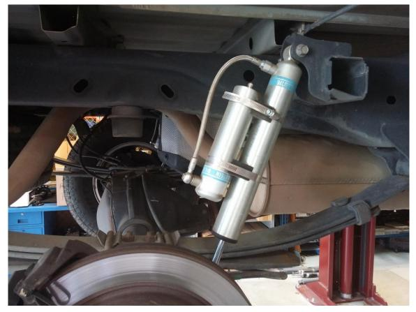
Figure 1. Reservoir placement for both sides
