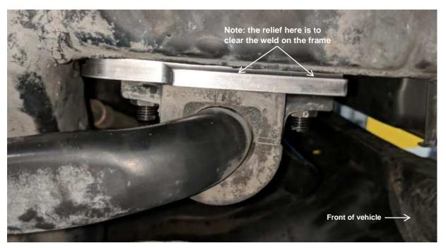
Z. Install the OE sway bar bracket as shown above and secure with the two Flange Nuts (BOM item # 17) using a 15mm wrench. Place a flat head screw driver into the slot in the end of the Flat Head Screw to keep it from rotating while tightening the Flange Nut.
