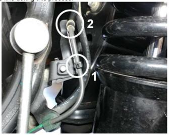
DD. Remove OE ABS line bracket by removing the hex head cap screw with a 10mm socket.
