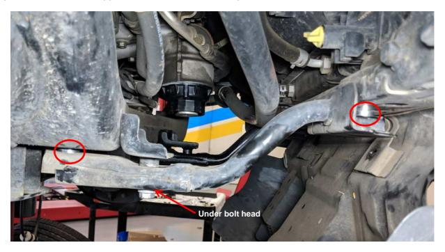
BB. Re-install skid plate with the bolts that were removed in step A (2 per side). **Torque skid plate bolts to service manual specification.**
