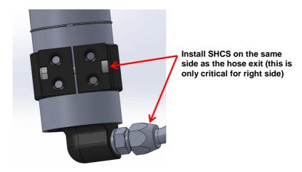
Q. Prepare the following assembly by applying non-permanent thread locker to two Flange Head Cap Screws (BOM item #6). Mount the Reservoir Clamp to the Reservoir Mount Plate (BOM item #12) as shown below using the two Flange Head Cap Screws. Tighten using a 13mm socket.
