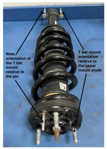
Figure 1: OEM T Bar/spring clocking.
