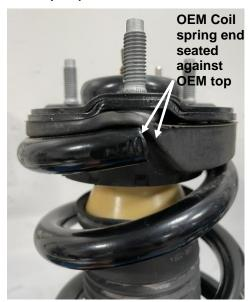
Figure 3: OEM Coil spring clocking.
