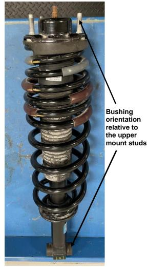
Figure 1: OEM Bushing/spring
