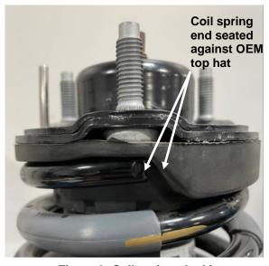
Figure 3: Coil spring clocking
