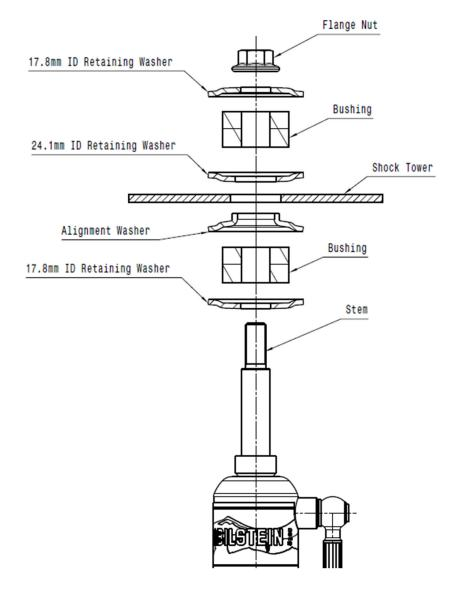
Figure 4. Bilstein Upper Stem Hardware Assembly
