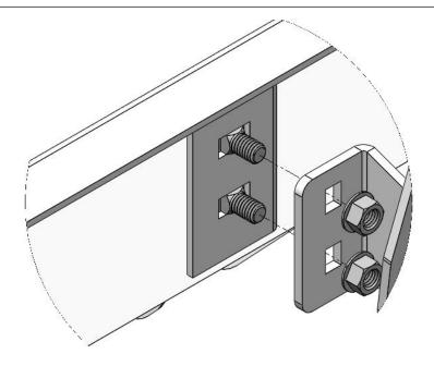
**<u>Step 3:</u>** Starting with the Driver Side. Remove all 8mm flange nuts from the 8mm factory threaded studs to remove the OE running boards.
