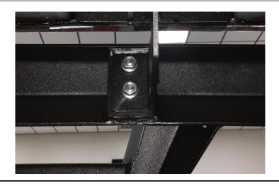
**<u>Step 7</u>**: Adjust the step rail to where you have approximately ¼" gap between the body of the vehicle and the top of the rail.
