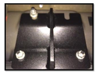
**Step 6:** Next, adjust the step assembly up/down and front/back to level out the step rail with body panel and then tighten step to brackets at 30 ft. /lbs.
