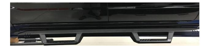
**<u>Step 8</u>**: After finial adjustment, tighten all rocker panel brackets to 30 ft./lbs.
