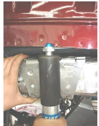
16. With airbumps installed in can, Cycle suspension with tires on and off up and down and make sure this is the correct location and nothing is making inappropriate contact. This is your last chance to make sure it is correct.
