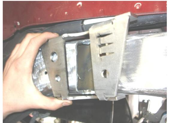
13. Reinstall bracket around frame rail inline with cut/marks and place bumpstop in correct position inside cut/bracket.
