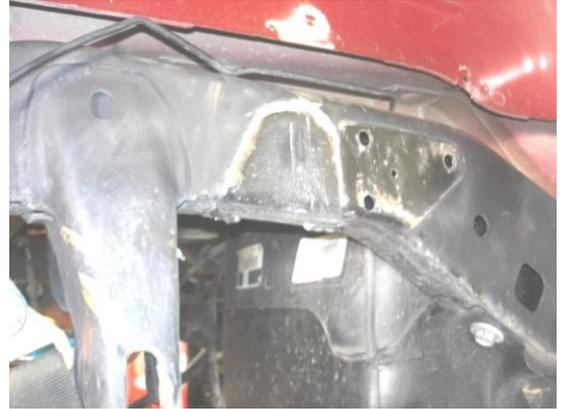
10. Line up the bumpstop in bracket and center plate and bumpstop in bracket centered up on bumpstop pad on axle.
