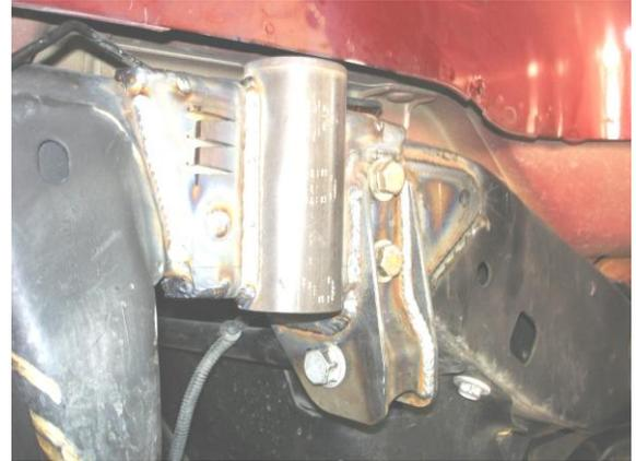
17. Once deemed correct location, remove airbumps, weld completely around brackets on frame and onto airbump tube.
