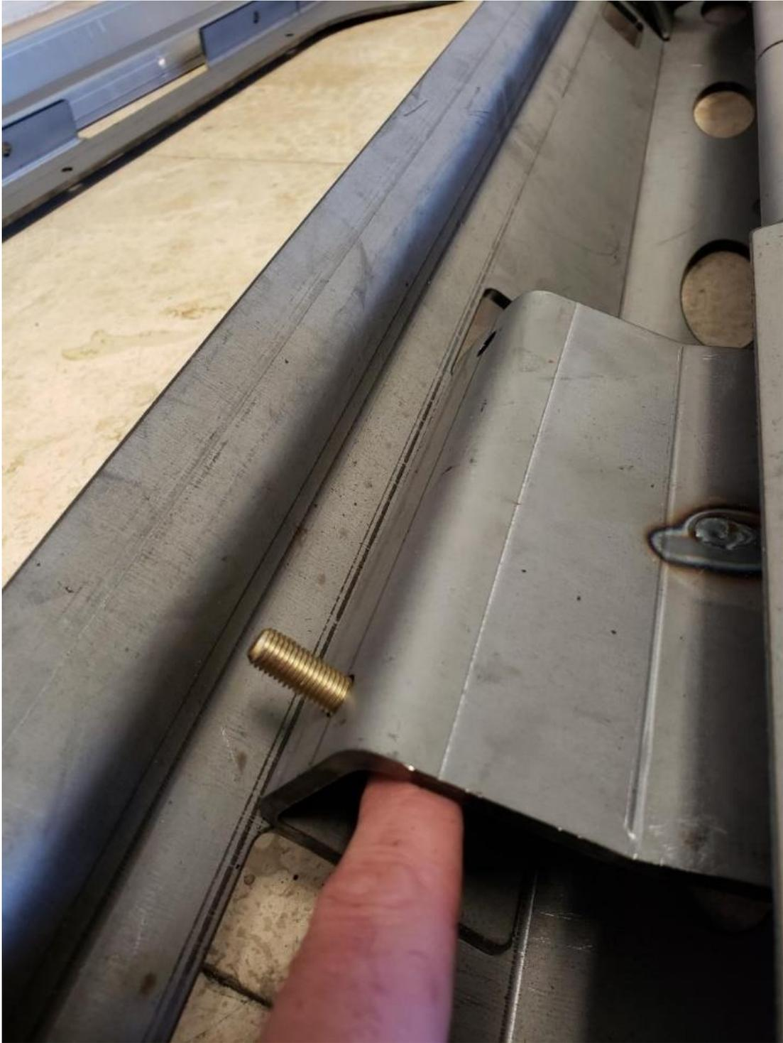
7. Insert the supplied crush tube at the front body mount. Between the Bomber Rocker and the body mount. Loosely (just before tightening) install the supplied M12 bolt with washer at this front body mount.
