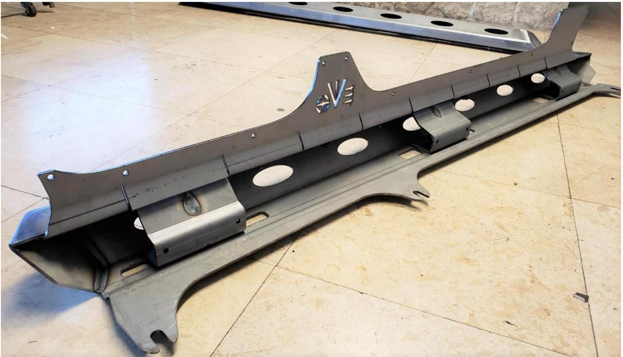
6. Using supplied 5/16" Hex bolts with washers. Install through inner seam mount at most forward and most rearward location. We suggest applying a layer of protective tape on the upper edges of Rockskin panel. With the help of 2 people, lift Bomber into location and insert front and rear bolts into existing pinch seam holes at body. Loosely install washer and nut. This will loosely hold part into place.
