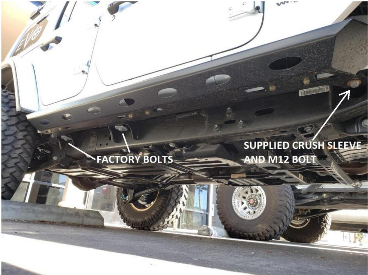
9. Using a jack, apply an upward and inward pressure to the bomber rail, lifting it up to an approximate level/as installed location. Lift until the assembly/rockskin match bodyline. Tighten all the 5/16" button head bolts.
