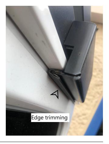
11. Insert bolt and washer from top down of upper mounting plate and thread into outer rail mount. Lower edge with trim should be grabbing underside of hardtop drip rail.
