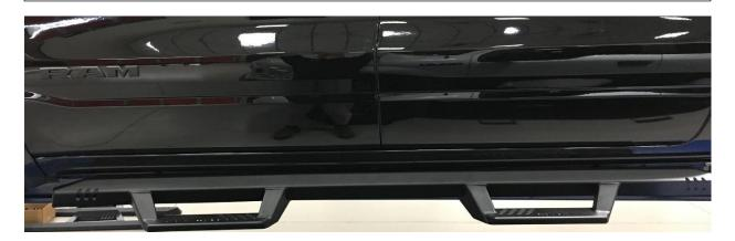
**Step 8:** After finial adjustment, tighten all rocker panel brackets to 30 ft./lbs.
