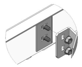
NOTE: Larger bracket will attach towards the front of step rail in the first position.
