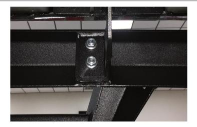
**Step 7:** Adjust the step rail to where you have approximately ¼" gap between the body of the vehicle and the top of the rail.
