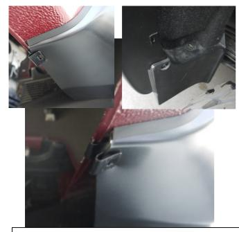
**STEP 17:** Slide the top edge of rear front mudguard cut out behind the factory mudguard. Install the E shape clip so that the clip slides over the inner sheet metal lip and is in line with the slot in the underside of Fender Flare. To secure the clip to Fender Flare apply inward tension on Fender Flare to the vehicle fender when installing the E clip, position the clip so that the barb in the clip locates in the slot of the Fender Flare.
