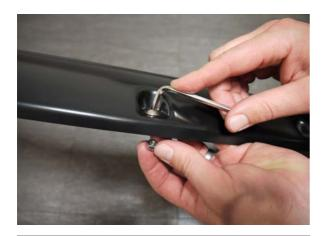
**STEP 1:** Attach the 10 bolts and nuts to each Fender Flare using a 3/16" Allen key and a 10.0mm wrench/socket. (wrench /socket and Allen key not supplied). Ensure inside of Fender Flares where the rubber seal is attached is clean, using the alcohol wipes provided. Wipe away any residue with a dry clean cloth.
