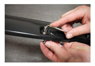
**STEP 11:** Attach the 12 bolts and nuts to each Fender Flare using a 3/16" Allen key and a 10.0mm wrench/socket. (wrench /socket and Allen key not supplied). Ensure inside of Fender Flares where the rubber seal is attached is clean, using the alcohol wipes provided. Wipe away any residue with a dry clean cloth.
