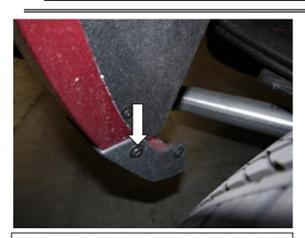
**STEP 15:** Using #15 Torx head screwdriver remove upper screw from the rear factory mudguard. Maintain screws for re-install.
