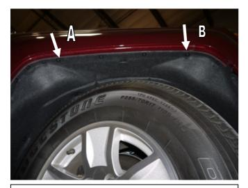
**STEP 5:** Place Fender Flare on the vehicle into the position of best fit. Note where the slots in Fender Flare at positions **A** and **B** align with the existing screws in the vehicle wheel arch. Remove Fender Flare. Remove the existing vehicle screws in location **A** and **B** using #15 Torx head screwdriver. Maintain screws for re-install.
