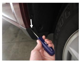
**STEP 6:** Using #15 Torx head screwdriver remove upper screw from the front factory mudguard. Maintain screws for re-install.
