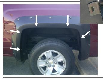
**STEP 16:** To secure the Fender Flare to the body, apply upward tension on Fender Flare to the vehicle fender when installing the black metal clips. Slide the clips over the Fender Flare and the inner wheel arch lip in the five locations shown. Position the clip so that the barb in the clip locates in the slot of the Fender Flare.
