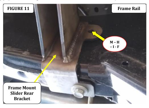
**Step-9** Align the Frame Mount Slider with the vehicle and tighten all bolts securing the Frame Mount Slider to the front and rear. Remember to check and retighten the nuts and bolts every six months.
