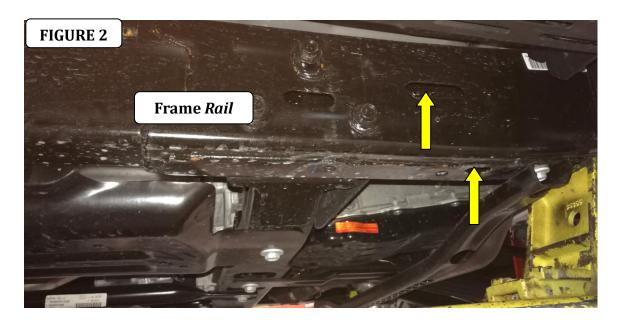
**Step-2** At the front location, thread a bolt plate in the guide bolt then introduce it through the obround hole, the tip of the bolt guide must come out through the bottom hole of the frame rail. Do not pull out the bolt plate attached to the bolt guide. Place another bolt plate in the obround hole and use a vinyl gasket to prevent the bolt plate from falling into the frame rail, (FIGURE 3 & 4).
