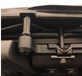
Pull the top all the way back and attach the rear strap to the hole in the back of the roll bar. Tighten the strap until snug.
