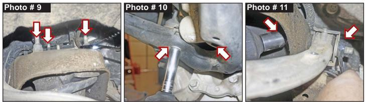
15. <u>Note</u>: Skyjacker UCA are Side Specific: Part number is on silver bar code label: # GM1935UCA-L Driver & # GM1935UCA-R Passenger. Install Skyjacker UCA to appropriate side of vehicle. Align the location of the OEM alignment cams with OEM hardware using a 21mm socket \ wrench. (See Photo # 12)
