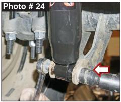
Install Skyjacker ADX rear shock. Connect upper shock mount with OEM hardware using a 21mm socket \ wrench. Connect lower shock mount with OEM hardware using a 21mm socket \ wrench. Secure, but **Do Not Completely Tighten** at this time.
