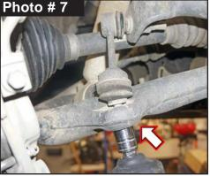
11. Support the bottom of OEM steering knuckle with jack. Loosen, but do not remove upper OEM ball joint nut from OEM knuckle using a 18mm socket \ wrench. (See Photo # 8) To unseat upper OEM ball joint taper, strike ball joint boss of knuckle using ball peen hammer to dislodge. <u>Note</u>: ONLY strike knuckle portion only. Remove nut & remove ball joint from knuckle. <u>Tech Note</u>: You may need to pry upper control arm down to disconnect ball joint.
