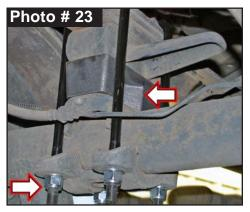
7. Install Skyjacker 9/16" U-Bolts over OEM top plate\leaf springs down into OEM u-bolt plate. Install supplied 9/16" Nylon Insert Nuts using a 7/8" socket\wrench. (See Photo # 23) Torque u-bolts evenly using an 'X' crisscross tightening sequence. Torque 125 ft.-lbs.
