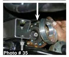
56. Hold the new Skyjacker front differential skid plate in place with the mounting holes of the new skid plate facing the rear of the new front & rear cross members. Using a hammer & punch, mark the four mounting hole locations. Drill the marked mounting location holes, using a drill & 5/16" drill bit. Using the four supplied 5/16" x 1" bolts, eight 5/16" washers, four 5/16" nuts, a 1/2" wrench, & 1/2" socket, install the new front differential skid plate. (See Photos # 36 & # 37)
