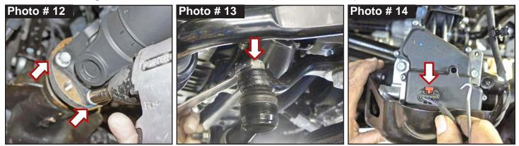
21. Connect wiring harness to passenger side OEM front upper control arm.
