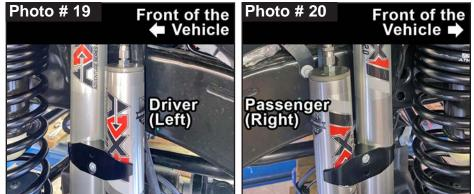
Install Skyjacker ADX front shock with OEM hardware at upper shock tower mount using a 18mm socket \ wrench. <u>Note</u>: Upper shock mount has a OEM fixed nut welded onto frame. Be careful not to dislodge nor over tighten this nut.
