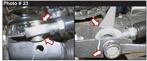
wheel to align track rod end with mount.
