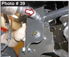
16. Coat supplied # HG58125-K Hourglass Bushing with a water resistant grease & press into upper & lower mounts of Skyjacker # SBE507-L Rear Sway Bar End Links. Coat & press # 403712 1.50 Long Steel Sleeves into upper & lower mount bushings.
