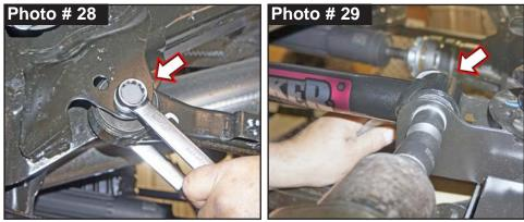
One at a time, install Skyjacker # GULR24-SX-L Rear UCA with OEM hardware using a 21mm & a 24mm socket \ wrench. (See Photo # 29)
