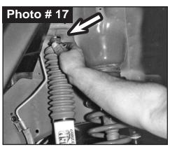
Loosely assemble two (2) supplied reservoir clamps with two (2) supplied hex head bolts using a 5/32" Hex Key socket. Position clamp into place around shock & reservoir cylinder. Secure, but **Do Not Completely Tighten**.
