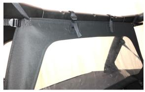
Hook both straps on the bottom of the Windbreaker to the floor hooks and tighten.
