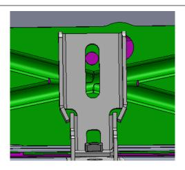
**Step 3:** Using the supplied M8x25mm hex bolts and washers begin hand tightening both upper and lower mounts to the rear two brackets.
