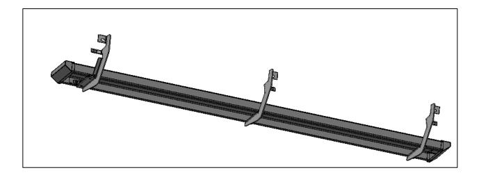
**<u>Step 7</u>**: Insert the supplied threaded brackets (x3) inside the running board lip over the top of each bracket.
