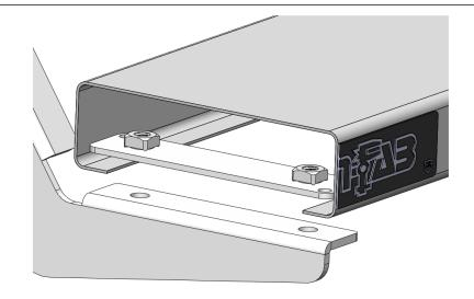
**<u>Step 9</u>**: After final adjustment, tighten all running board threaded mounts. **<u>Step 10</u>**: Next, tighten the lower pinch weld attachment points (x3). **<u>Step 11</u>**: Finish by tightening the upper mounts (x3).
