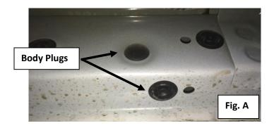
**Step 3:** Using the measurement from the brackets, only remove the rubber plugs from the sections you will need to mount the step. (**NOTE**: Start with the first section nearest to the front of the vehicle.)
