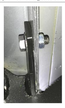
**Step. 6:** After finial positioning, completely tighten all (x6)  $\frac{1}{2}$ " -20 x  $\frac{3}{4}$ " in the pinch weld attachment.
