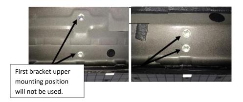
**Step 3:** Position step up to the body of the vehicle and align the brackets up with the factory mounting locations.
