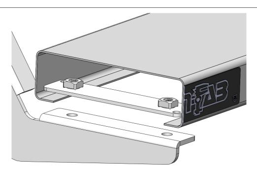
**Step 8:** After final adjustment, tighten all running board threaded mounts.
