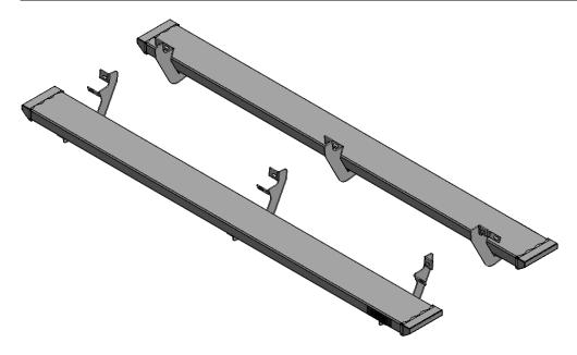
**Step 1:** Beginning with the driver side, remove any factory running boards or steps and discard.
