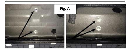
**Step 3** Starting with the driver side, position Trail slider up to the body of the vehicle and align the brackets up with the factory mounting locations.
