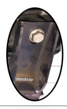
Use factory body mount bolts. \*\* Front mount does not use the factory bell washer \*\*\*
