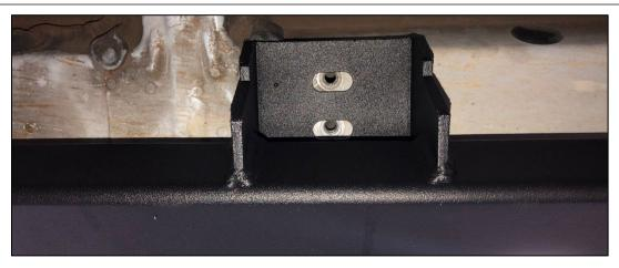
**Step 5** Start all remaining M8x30mm hex bolts in each bracket and leave loose.
