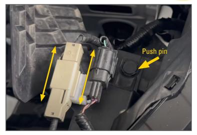
Step 4. Remove the (2x) plug connectors located to the left hand side corner of grill.
