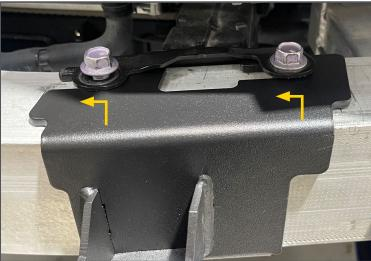
Step 32. Install factory bolts in bottom bracket and tighten to factory specs.
