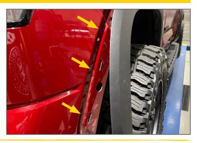
Step 10. Once you have separated fender trim, pull plastic portion of bumper away frommetal fender.
