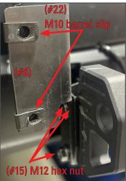
Step 37. Level upright bracket and tighten hardware to (65 ft-lbs). Repeat step with opposite side.
