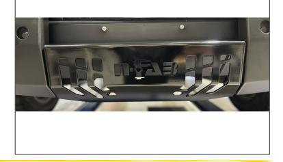
Step 44. Confirm that light hoop and skid plate are in alignment and fully tighten (4x) up right bolts to (32 ft-lbs). Step 45. Install #16 (4x) locking panel plugs in uprights to cover hardware. If parking sensors were not relocated, install #17 (2x) locking panel plug to cover sensor hole.
