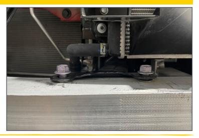
Step 31. Install #8 driver side mounting bracket in between factory frame bracket and crash bar.
