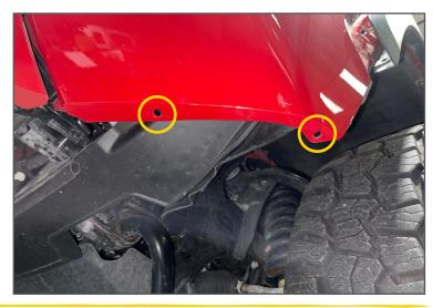
Step 8. Remove the bottom (4x) 10mm bolts that attach the grill to the crash bar.
