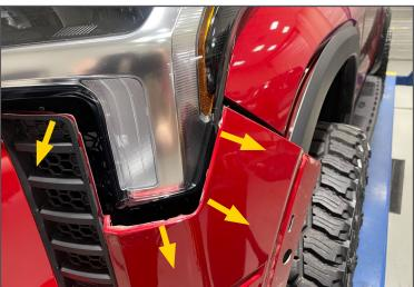
Step 11. From center of grill, lift bumper up, out, and away from vehicle. Your bumper will come out in one piece.
