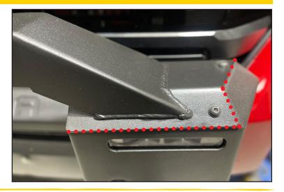
Step 43. Install #4 skid plate using #11 (4x) M8x20mm flanged hex bolt and #18 (4x) flanged hex nut. After final adjustment, tighten hardware to (20 ft-lbs).
