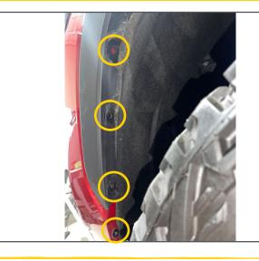
Step 7. Remove the bottom (2x) 10mm bolts from fender.
