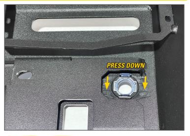
Step 20. Install #14 (2x) M6x20mm hex bolt with #21 (2x) push nuts in the designated fog light bracket holes. Repeat steps with driver side upright.
