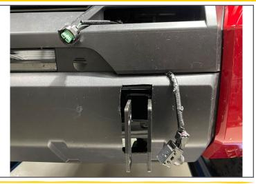
Step 35. Install #5 tow hook and #6 driver side vertical mount plate using the supplied #15 (3x) M12x55mm hex bolts and #24 (3x) M12 flanged hex nuts. Step 36. Install #22 (2x) M10 barrel clip nuts.
