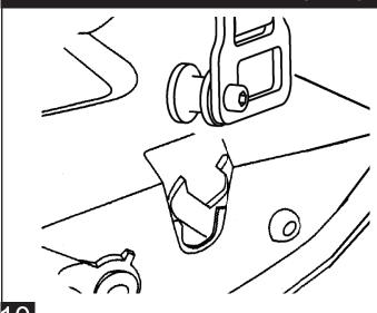
When the BEDXTENDER is at the furthest rear position, push down on the buckle to insert into tailgate latch. Tighten straps. To release, pull tailgate handle.
