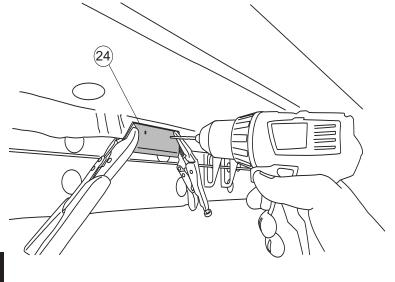
With drill template secured with vise grips, drill 1/8" Pilot holes. Remove template and drill holes to 21/64".
