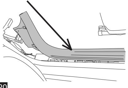
Reinstall the drivers side door sill trim-panel, be careful to not damage or pinch the wires.
