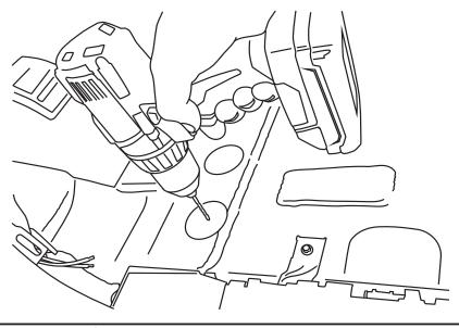
Lift the carpet to expose the plastic in-floor plug. Drill a 9/32" hole in the middle and insert the supplied rubber grommet (22).
