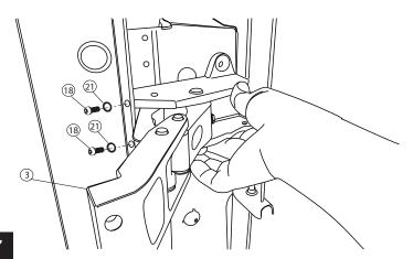
Install rear linkage (3) to the pinch weld using the supplied M8 button head bolts (18) and M8 washers (21).
