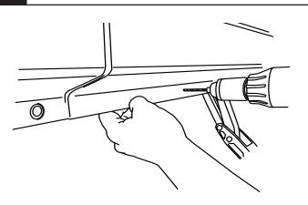
Center punch and drill a 1/8" pilot hole then drill a 9/32" hole through the pinch weld at marked locations. Deburr all holes. After drilling apply paint to holes to prevent rusting.
