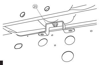
Snug the front linkage bracket (25) to the rivenut first. Note: bracket to be oriented closest to the frame.
