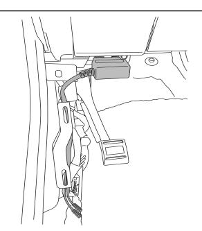
Next plug in the OBD module under the dash as shown and route the wires behind the bracket to the left. The wires from below can be tucked under the carpet for the trim to be installed on top. Make sure the wires are clear of the E-brake mechanism.
