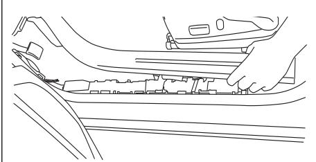
Remove the drivers side door sill trim-panel, by pulling up and back.
