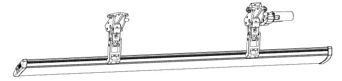
Line up the front edge of the board just behind the front fender trim. Repeat on passenger side. Torque the bolts to the step extrusions to 10 ft-lbs(13.5 N m).
