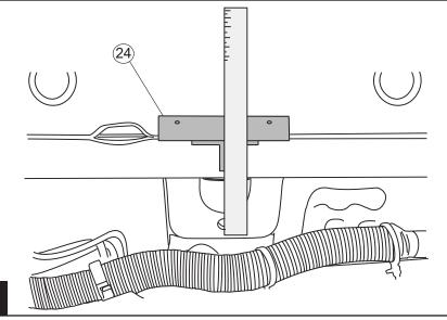
Place tail of drill template (24) on the inner rocker surface and slide it until the template rests on the outside of the pinchweld. Use a straight edge as shown to line up the center of the template with the center of the mounting hole in the body crossmember.
