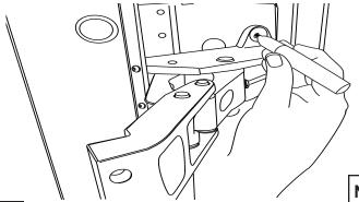
The **rearward tab** on the linkage upper mount will land on the body crossmember, mark the center of the hole and remove the linkage. (Crew Cab Only)
