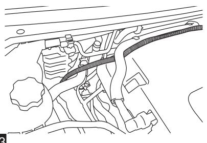
Route the passenger harness-leg down to the outside of the frame on the passenger side behind the inner fender liner, over the body mount bracket and to the motor on the front linkage. Secure with zip ties.
