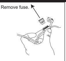
Remove Fuse from harness. Plug harness to controlle. Attach controller horizontally to driver side wire loom. Secure with 11" cable ties. Attach ground lead to the negative battery terminal. Open the power distribution block cover and connect the Power wire to the positive power battery cable terminal.
