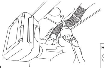
Enlarge the hole on the front body support member. Hole is located approx. 29" from front fender edge. Use a 17/32" Drill bit. Install a rivet nut (20) using the supplied rivet nut tool (19).
