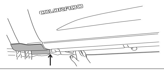
Front & Rear Linkages on Driver and Passenger side: Torque fasteners to 16 ft-lbs. (22 N m).
