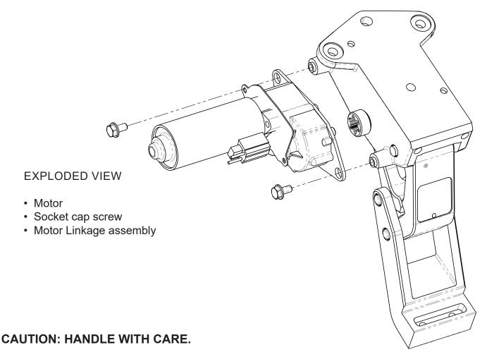
To ensure our customers receive all components with full integrity, we pack the motors separate from their Linkage assemblies. This requires that the installer position and fasten the motor before continuing with the install. Please follow the instructions below and handle the assembly carefully.
