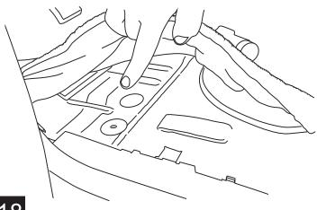
Pull the yellow trigger wires through the grommet from below. Use the Posi-Lock™ (11) to make the connection to the plug and play module.
