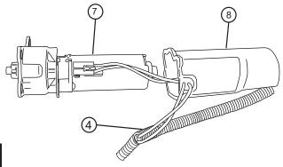
Insert plastic push pin rivets (13) in mounting holes of motor cover (8). Use pliers to ease installation.
