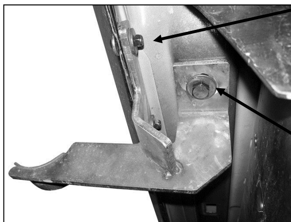
(Fig 3A) Passenger side Front Mounting Bracket installation pictured ("mid length" bracket)
