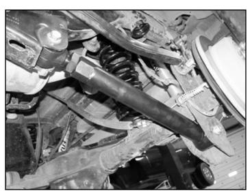
HINT: If mounting bolt is difficult to install due to misalignment of Control Arm bushing with mounting bracket, either (1) adjust height of axle housing with hydraulic jack, (2) move axle housing into position with a heavy-duty ratchet strap, or (3) temporarily disconnect track bar until mounting holes align.
