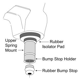
Cut away the lower portion of bump stop holder until even with bottom of flat washer. DO NOT CUT OFF FLAT WASHER! HINT: A die grinder with cutoff wheel or reciprocating saw is useful for cutting bump stop holder.
