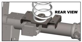
IMPORTANT: Adjustable Spring Mount bracket must be installed with rounded side facing forward and flat side facing the rear as illustrated above.
