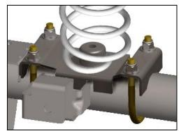
O Using a torque wrench, tighten U-bolt nuts to 50 ft-lbs.
