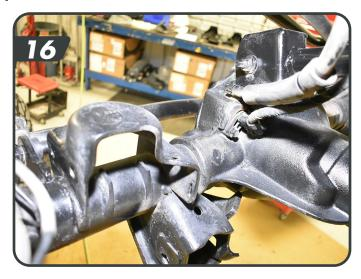
Using a cut off wheel cut the LCA mount flange of the axle as shown. [17]
