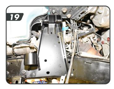
(3.6L ONLY) Remove the forward factory fastener holding the heat sheild to the motor mount bracket. Mount the frame to coilover back support bracket to the factory motor mount bracket with the provided 3/8" bolt, nut and washer in bolt pack J137. Leave hardware loose[20]
