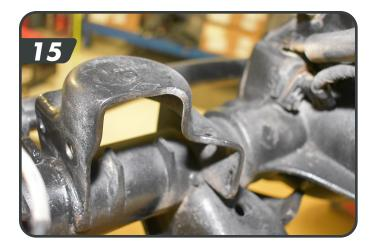
Using a small (3") cut off wheel or Recipricating saw cut the shock mount off of the axle as close to the axle as possilbe without hitting the axle. [16]
