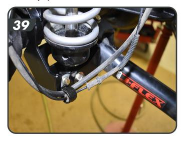
h. Reattache the factory brake line to the frame through the frame mount with OE hardware (10mm). Torque Bolt to 115 in-lbs.
