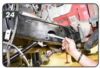
h. One at a time remove each ½" bolt and use the provided loctite. Torque the steering box bolts (18mm) to 99 ft-lbs and the ½" hardware (¾" to 90 ft-lbs. Leave the brake line bracket bolt loose.
