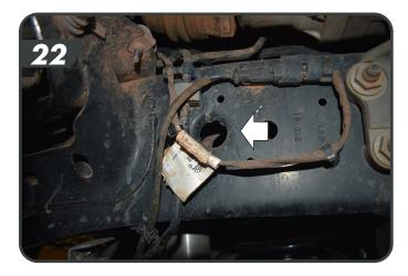
g. Insert the Long single nut tab [23, 24] into the frame from the outside large frame hole. Use the provided ½" hardware hold it in place. Leave loose.
