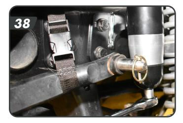
g. Using the provided 1/4" Hardware (7/16") in bolt pack J136 and the Hose Clip. Fasten the brake line and ABS line to the axle mount to prevent it from rubbing. Torque to 86 in-lbs (7/16" wrench and socket). Cable ties are also provided to attach the brake line to the abs line. [39]
