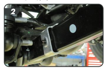
Disconnect the brake line from the Axle coil mount location [3] Remove the Axle bracket and LCA bracket from the brake line.
