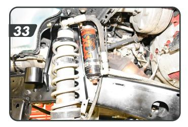
Raise the axle to mount the coilover into the lower mount. Fasten with the  $\frac{1}{2}$ " x 2- $\frac{3}{4}$ " bolt washer and nut. [34]
