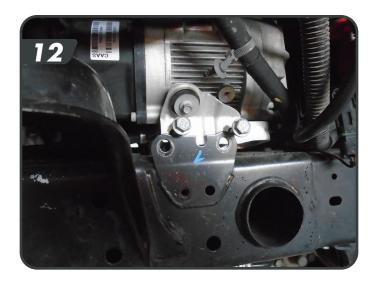
d. Grind the outside frame until smooth, Paint any bare metal. [13]
