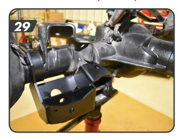
Mark the location of the most forward holes location on the coil mount. Remove the bracket and drill with a 7/16" Bit. Paint any raw metal.
