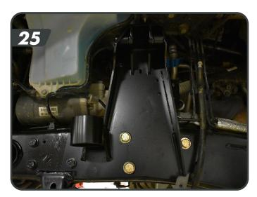
i. Mount the Frame to Coilover bracket support bracket to the Frame Mount Bracket with the Remote Resi Bracket using the provided 5/16" (½" socket and wrench) bolts, nuts, and Washers. [26] Torque hardware to 178 in-lbs
