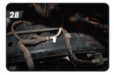
Ensure no brake lines or wires rub any of the new brackets or nut tabs and manipulate them out of the way as nessossary.
