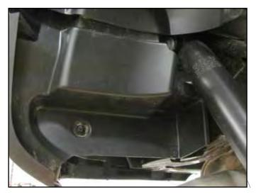
O Support the axle with a jack under the center of the differential and remove the shocks from the frame and axle and save hardware
