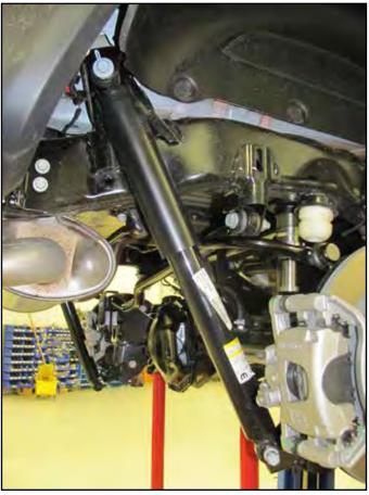
Cower the axle enough to remove the factory springs. Make sure there is adequate slack on all brake lines.
