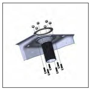
Once all 6 bolts have been installed, tighten the 5/16" Nylock Nuts (A) to 30 ft-lbs using a torque wrench.
