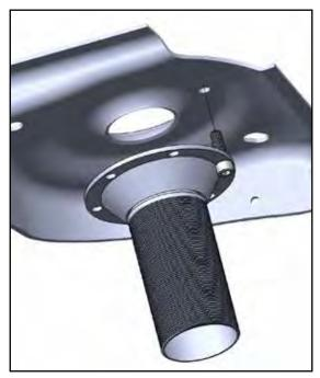
Using the Cone Adapter Plate (C) as a template, accuratly mark the 5 remaining hole locations on the upper spring mount.
