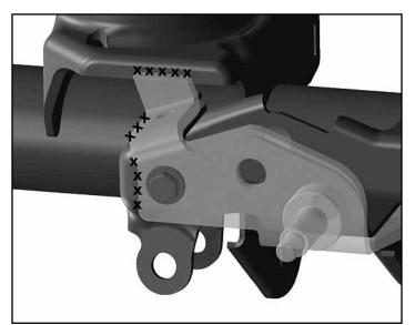
**HINT:** Be sure to include area on factory coil spring bracket and lower base of Relocation Bracket where it terminates just before it makes contact with axle tube.
