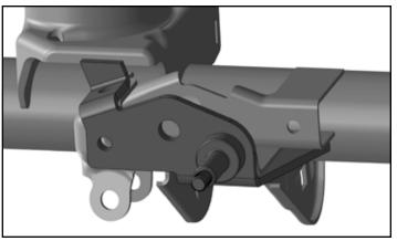
• Position the Relocation Bracket (A) against the factory track bar bracket as illustrated.
