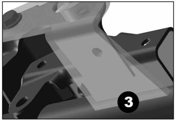
• Next, fillet weld Steering Stabilizer Relocation Bracket (A) to axle housing at all locations indicated by an "X" in step 2.
