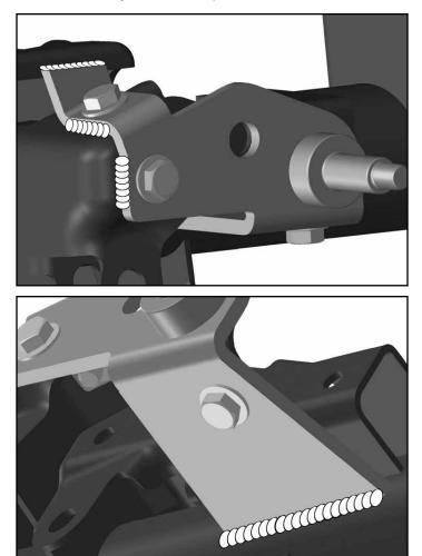
*IMPORTANT:* Avoid overheating axle tube and factory track bar bracket by welding a small section and allowing the surface to cool off regularly.
