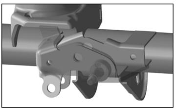
With the Relocation Bracket (A) in position, insert one 3/8" x 1" GR5 Bolt (B) with Flat Washer (C) into original mounting hole as illustrated below. Secure bolt with another 3/8" Flat Washer (C) and Ovalok Nut (D) and temporarily tighten to hold the bracket securely to the factory axle housing bracket.
