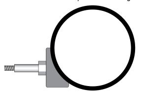
Carefully weld the Rear Axle Shock Mount to the axle housing, making sure the Hex Stud remains parallel with ground.
