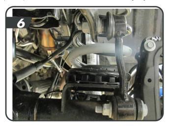
h. Remove the 4 bolts mounting the front driveshaft to the pinion flange (15mm). This is done to ensure the driveshaft does not bind when removing the coil springs. [7]
