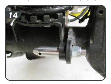
q. The kit comes with disconnect retention brackets to hold the links when the links are disconnected. Install the retention brackets using the provided 5/16" bolts into the factory hole in the front of the coil bucket [15]. These are designed to slightly interfere with the edge of the coil bucket to hold them in place.
