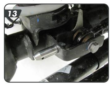
p. Install the longer disconnect post on the driver side axle sway bar link mount with it pointing inboard [14]. Fasten with the ½" nylock nut and tighten to 65 ft-lbs. Tighten the post with the pin hole parallel to the ground. Slide the polyurethane spacer on the pin up against the axle tab.
