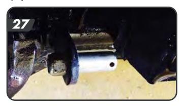
Note: In some cases a rotary grinder may be necessary to slightly open up the sway bar hole to clear the ½" bolt. This ensures a tight fit.
