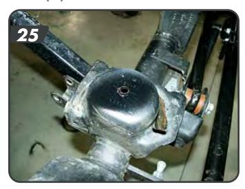
Place the provided bump stop extension inside one of the JSPEC front coil springs. Note: Taller springs are for the front. Install the front coil springs with the bump stop extension. Make sure the spring is seated properly in the axle mount.
