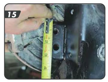
an. Re-install sway bar links into the drilled hole using the factory hardware. [16]
