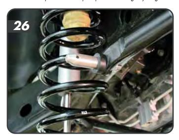
b. Remove the nut an install the lower mounting posts into the factory sway bar link holes so they are pointing inboard and the pin holes are parallel to the ground. The passenger side post is squared off to provide clearance between the post and the OE track bar bracket. [27]
