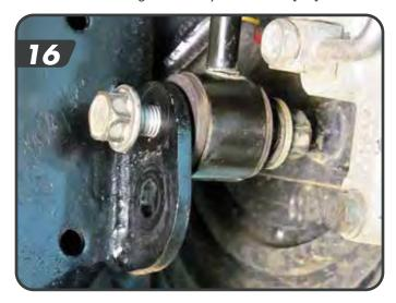
ao. Install the rear bump stop spacers on the axle with the 2" tall orientation for 2.5" lifts and 3" orientation for 3.5" lifts. In both cases the bump should be intalled with the offset in material forward. Fasten the bump stop spacer to the axle with the  $5/16" \times 7/8"$  bolts, nuts and washers. Torque bolts to 20 ft-lbs. (½") [17]
