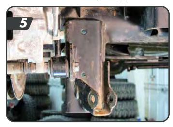
Lower the axle enough to remove the factory springs. Make sure there is adequate slack on all wires.
