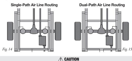
TO PREVENT THE AIR LINE FROM MELTING, MAINTAIN AT LEAST 6" (152MM) FROM THE EXHAUST SYSTEM TO THE AIR LINE.
