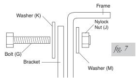
4. Install nut (J) and washer (M) on to the carriage bolt that was inserted through the jounce bumper bracket hole (Fig. 8).
