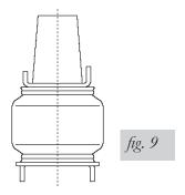
7. Tighten the upper bracket mounting hardware to 16 lb.-ft.
