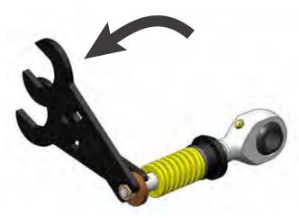
O Slide the spring off of the shaft.
