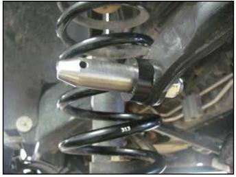
Note: Insert a small phillips head screwdriver or punch into the click pin hole to prevent the posts from rotating.
