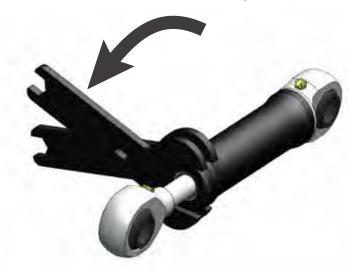
Note: If using a vice, put the cap in the vice jaws and use the provided wrench on the body to prevent the vice from binding on the threads.
