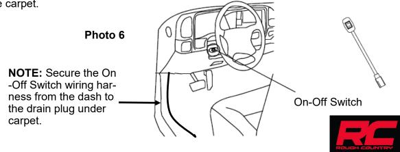
**NOTE:** Normal function of the On-Off switch once power has been connected to the positive and negative fused links on the battery. (On) the steps will extend for use and entering the vehicle. Steps will retract when both doors per side are closed connecting the magnet to the module. (Off) the steps will retract to the body of the vehicle even when the doors are open and the magnet is away from the module.
